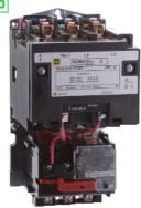
NEMA Motor Starter, Type S, nonreversing, Size 2, 45A, 25 HP at 460 VAC, up to 100 kA SCCR, 3 phase, 3 pole, Motor Logic, 208 VAC coil, open
